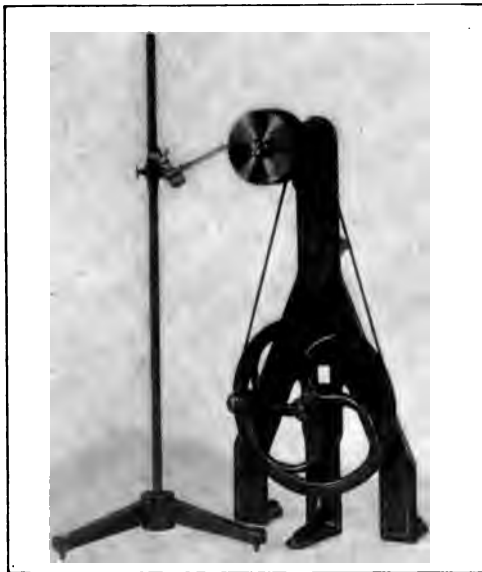
FIG. 24. Serrated disk for demonstrating the dependence of pitch upon frequency of vibration.
